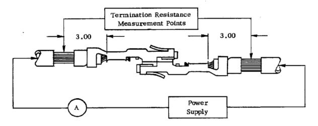
Notes: 1. A I foot minimum length of continuous lead for heat dissipation.
